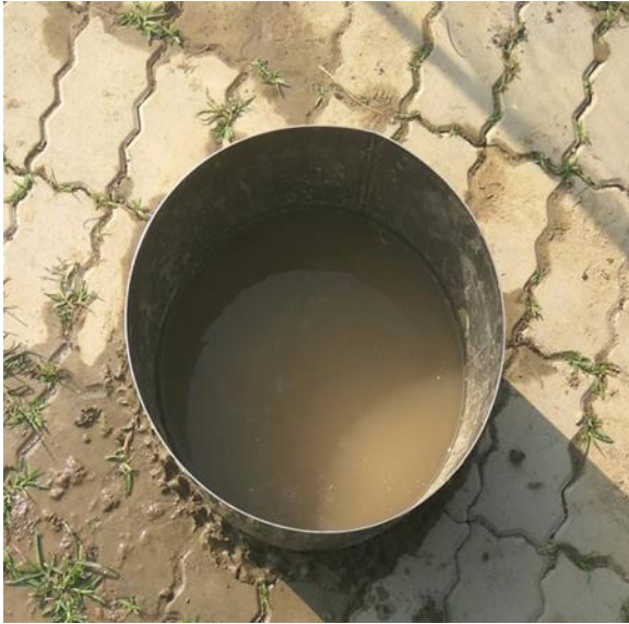
Fig (d) Double-Ring and single ring Infiltrometer of 20-40cm diameter of ring
