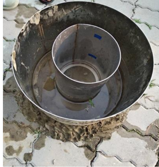
Fig (d) Double-Ring and single ring Infiltrometer of 20-40cm diameter of ring
